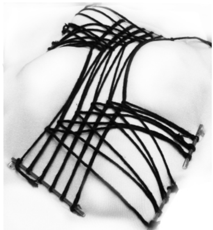
Inflated membrane is shaped by anchor threads
