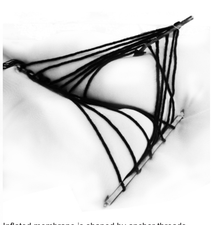
Inflated membrane is shaped by anchor threads
